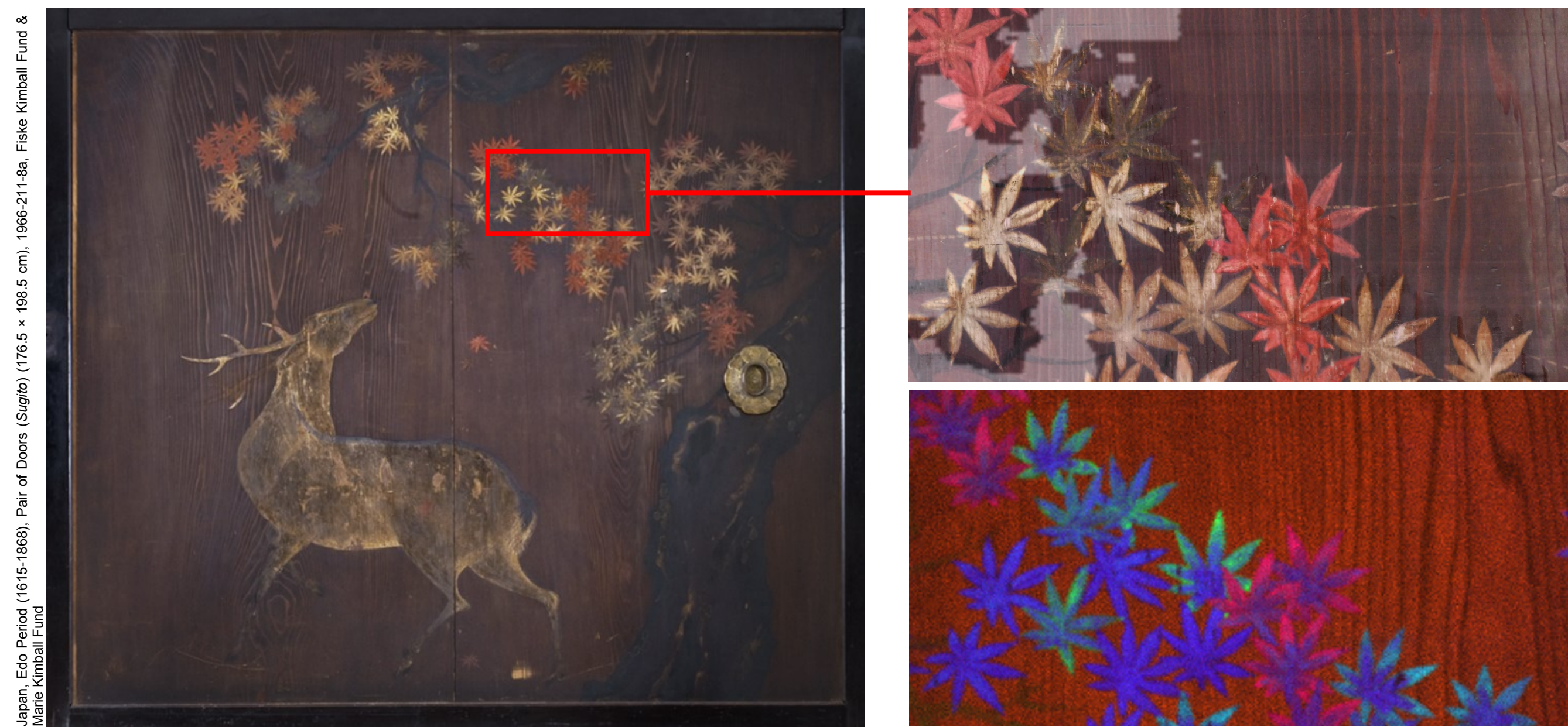
Figure 2. Left: Deer Under Maple Leaves . Right top: Detail of painted leaves in visible light. Right bottom: XRF false color map, revealing the selection & distribution of elements in colors of the autumn maple leaves: Hg (pink), Cu (green), Pb (blue), & Ca (purple).
