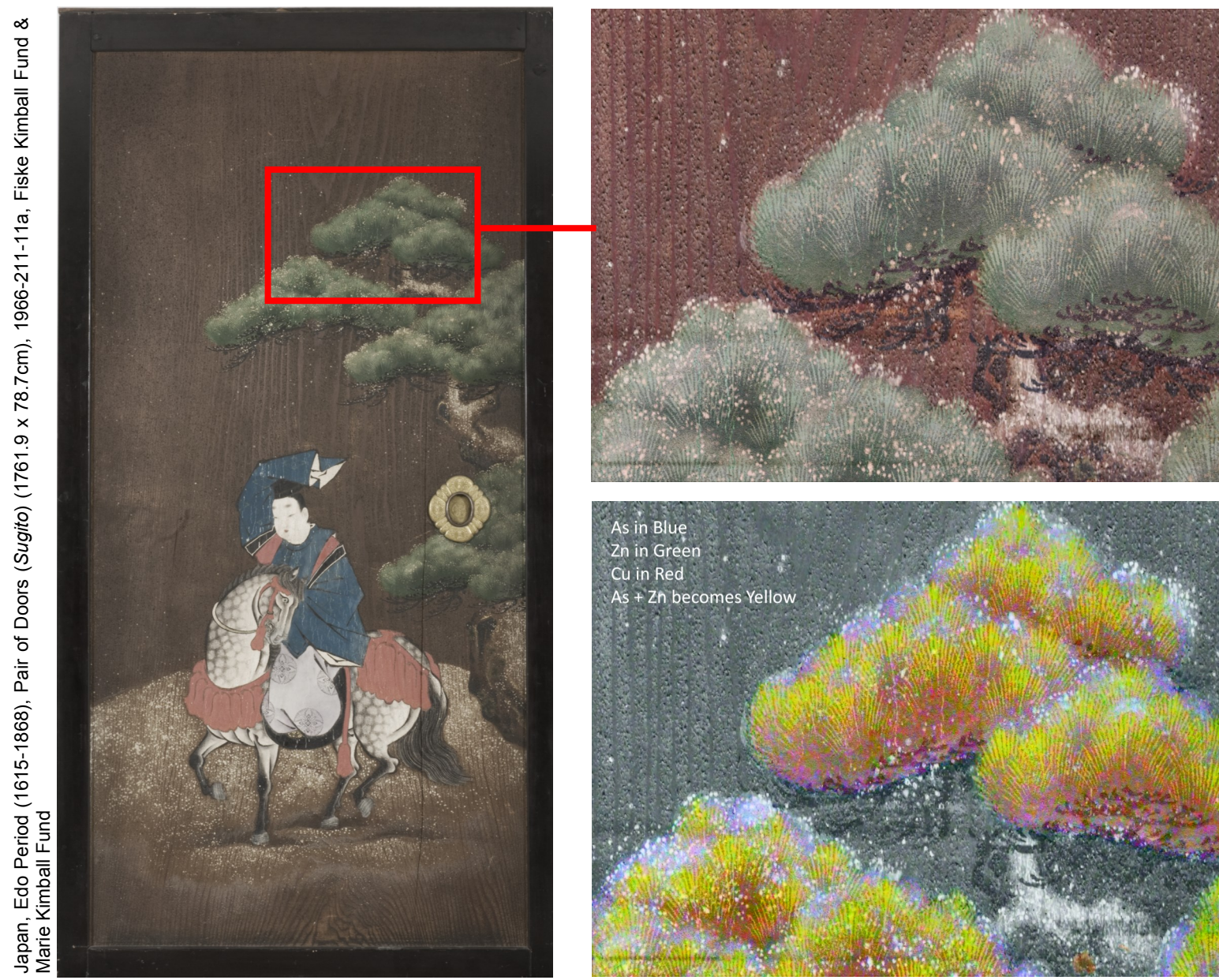
Figure 4. Left: Courtier on Horseback . Right top: Detail of pine tree in visible light. Right bottom: XRF false color map showing distribution of Cu (red), As (blue) & Zn (green) in green paint containing philpsburgite.
